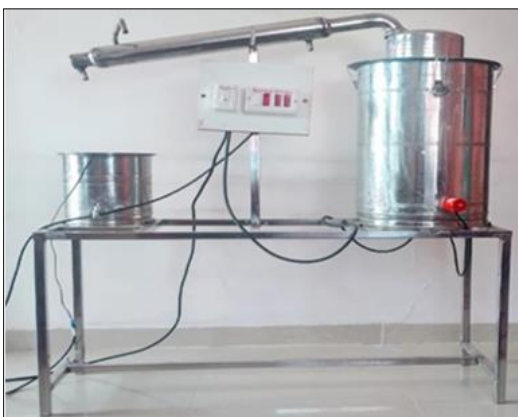
Fig 1: Experimental setup of steam distillation unit
